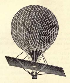
The accompanying illustration shows a plane for the above purpose fitted to a spherical balloon, which plane may be adjusted to any required angle.
